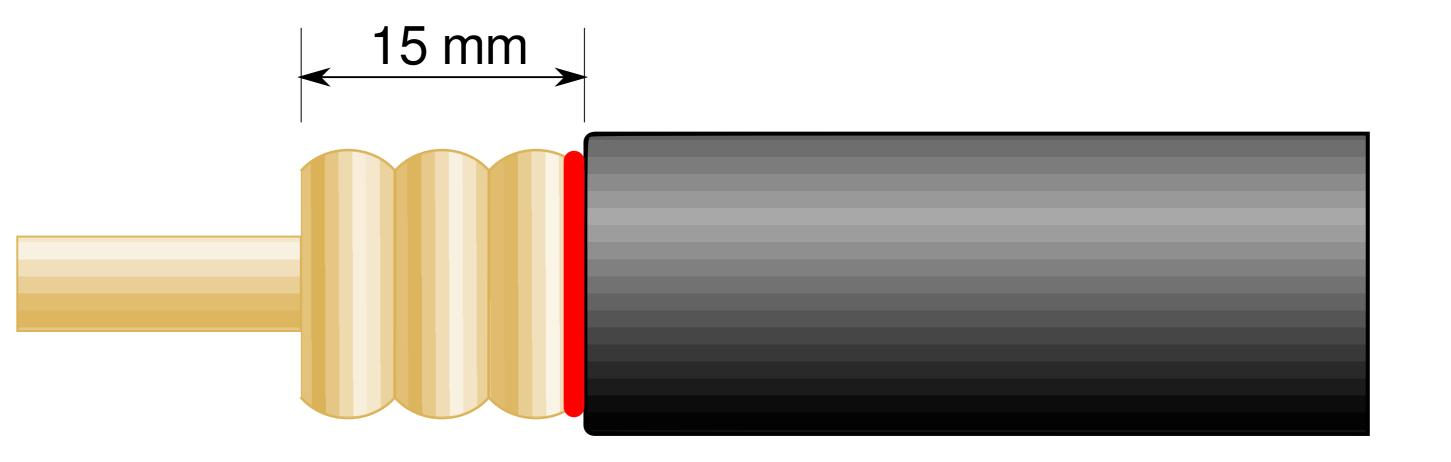
Cut the centre condutor so that 10mm is protruding from the dielectric. Ensure the end of the centre conductor is flat and clean of and debris or dielectric material
